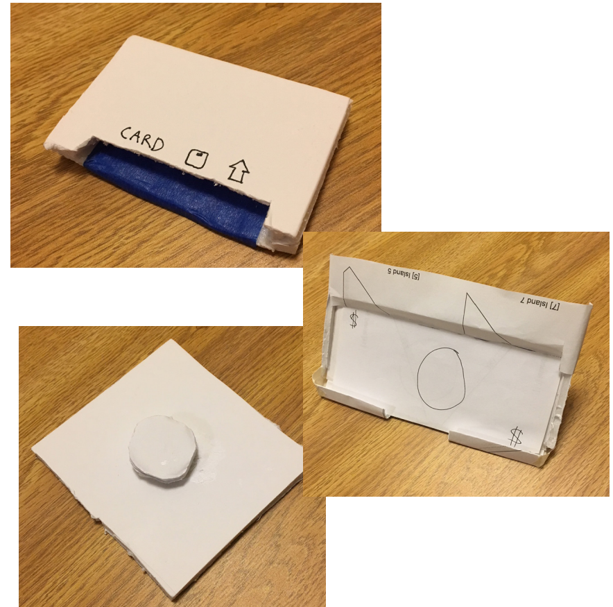
Some physical prototypes I created. They were built to demonstrate how the user was supposed to interact with the ATM on the small scale - inserting a card, retrieving money, and pressing a button.
